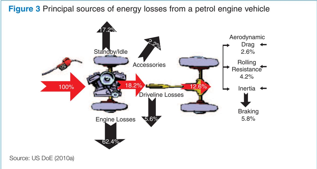
heat and idling. Further losses are caused by parasitic losses from accessories, and from the transmission (i.e. from delivering the mechanical energy created by the engine to the wheels) due to the number of rotating elements which incur friction losses. Ultimately, only a fraction of the energy that enters the engine is actually used to propel the vehicle forward.
