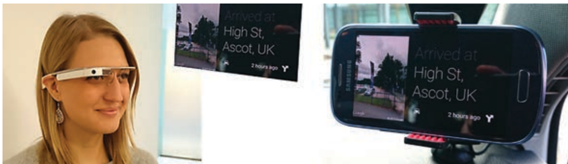
Figure 3: Smart glasses (left) and smartphone (right) both showing identical navigation information
