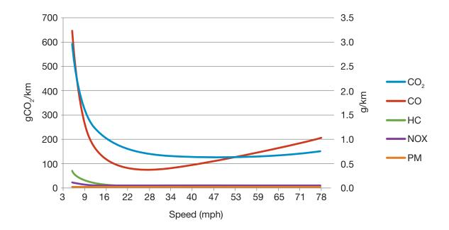
Figure 1: Pollutant emissions as a function of speed
