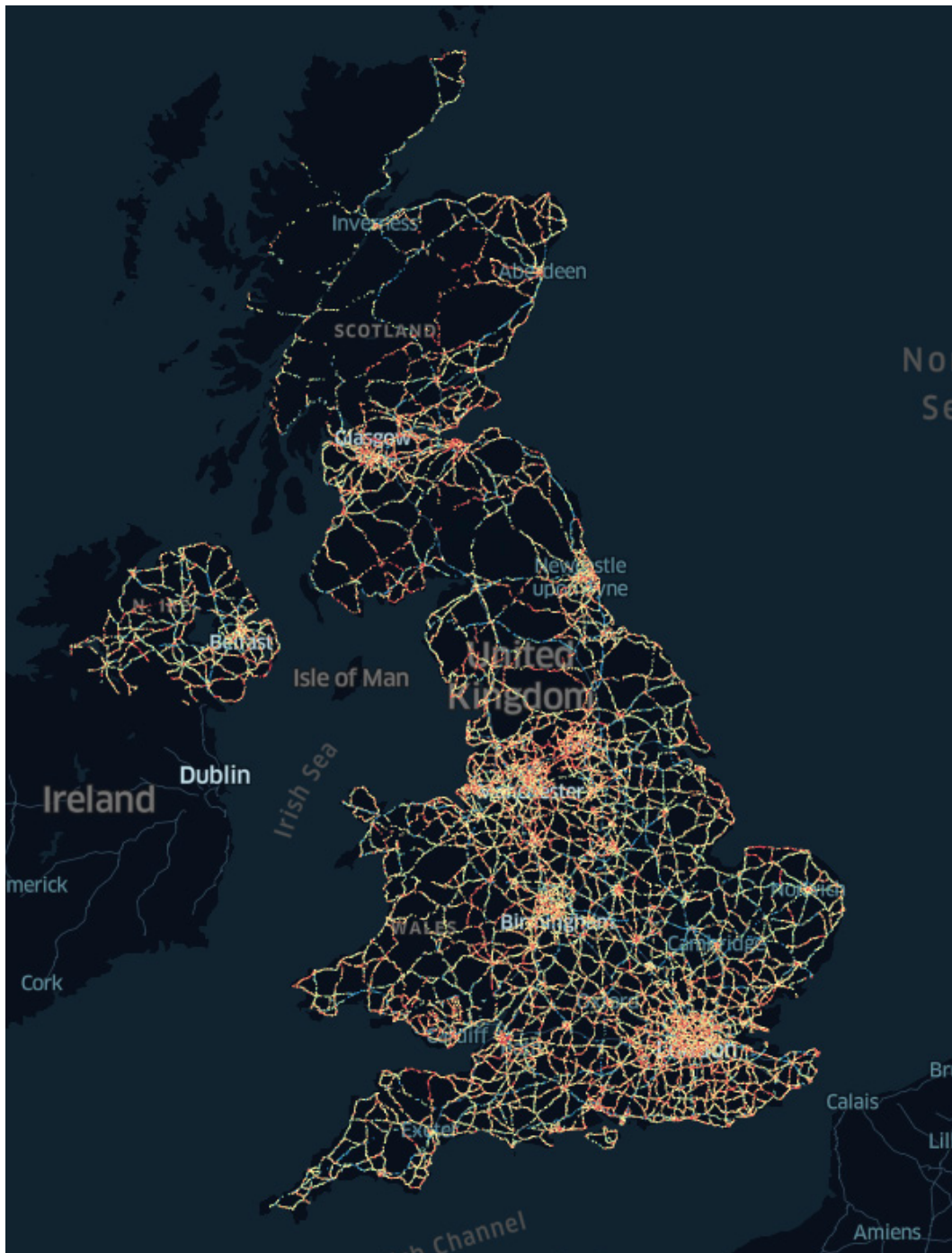
Figure 3.9: NIRA Dynamics Road roughness data for the UK, sourced from VW Group vehicles
