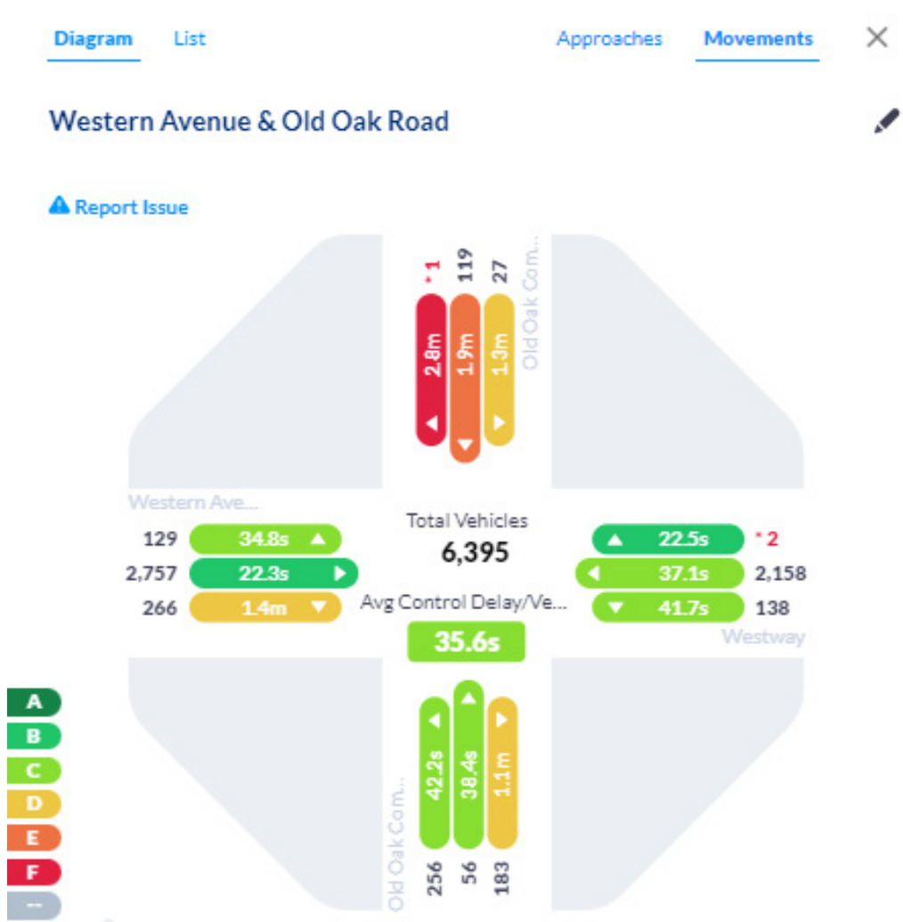
Figure 3.7: INRIX uses connected vehicle data to analyse traffic light performance
