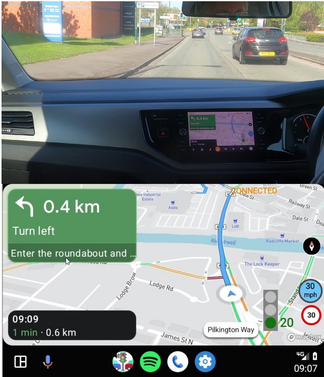
Figure 3.6: GLOSA integrated with navigation
