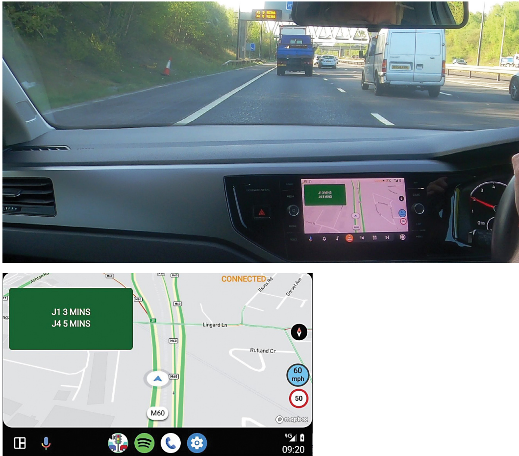
Figure 3.1: Typical IVS deployment – repeating journey-time signs on satnav
