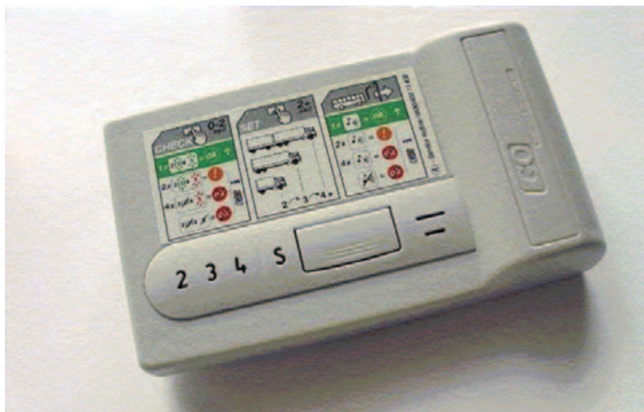
Figure 24: A microwave tag as used in the Austrian lorry tolling scheme
